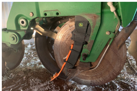
John Deere MaxEmerge planter, set out at 1m spacing, used for planting single skip dryland cotton.
